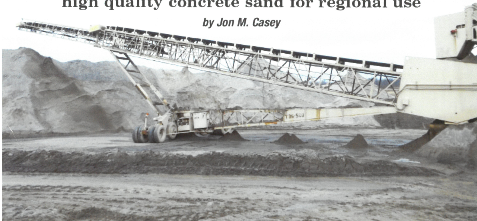
The THOR T36-500 telescopic radial stacker keeps concrete sand stockpiled, ready for customers.
