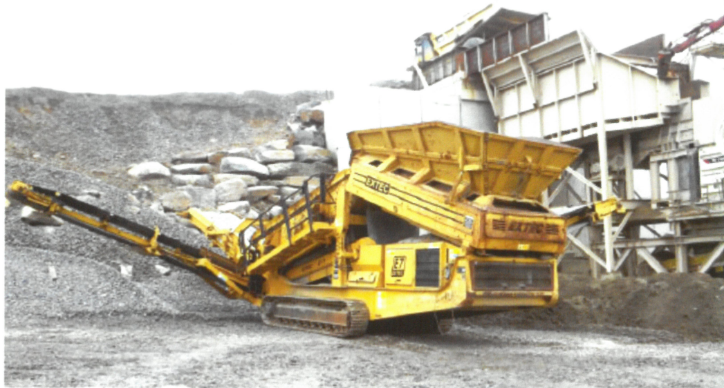
When the need arises, Pierson's crew uses this EXTEC portable screen plant to screen out ballast material.
