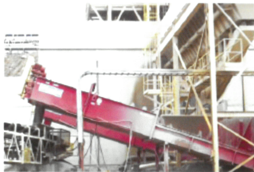
Twin McLanahan 44-inch sand screws process 200 tons per hour of material coming out of the Graystone 12 X 48 classifier.
