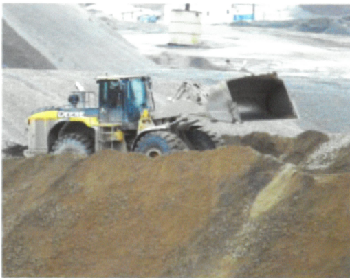
An operator moves ballast material onto a stockpile that could be used for snow and ice control.
